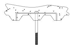
Before pouring concrete, locate the Figure 284 on deck so legs rest in "valleys" of form. Drill hole in deck for bolt.
